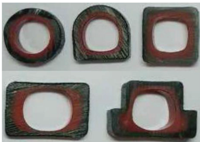
Figure 6. Cross-section of WAIM parts with different cavities. [30] Copyright 2016, Wiley-VCH.
