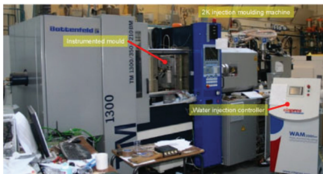
Figure 2. The commercially available water-assisted injection systems. Reproduced with permission. [19] Copyright 2008, Taylor & Francis.
